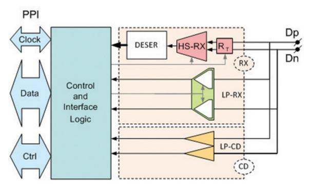
Figure 3: RX only configuration is quite smaller that a Universal lane, but cannot support full-speed production test
