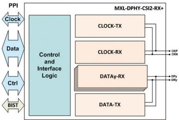
Figure 4: Mixel's RX<sup>+</sup> optimized configuration
