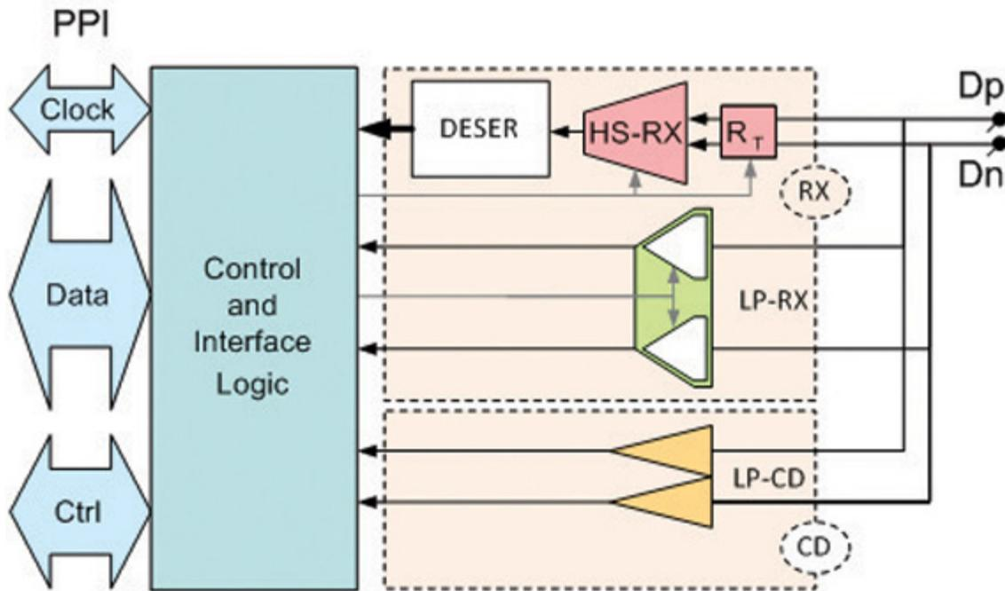
Figure 3: RX only configuration is quite smaller than a Universal lane, but cannot support full-speed production test
