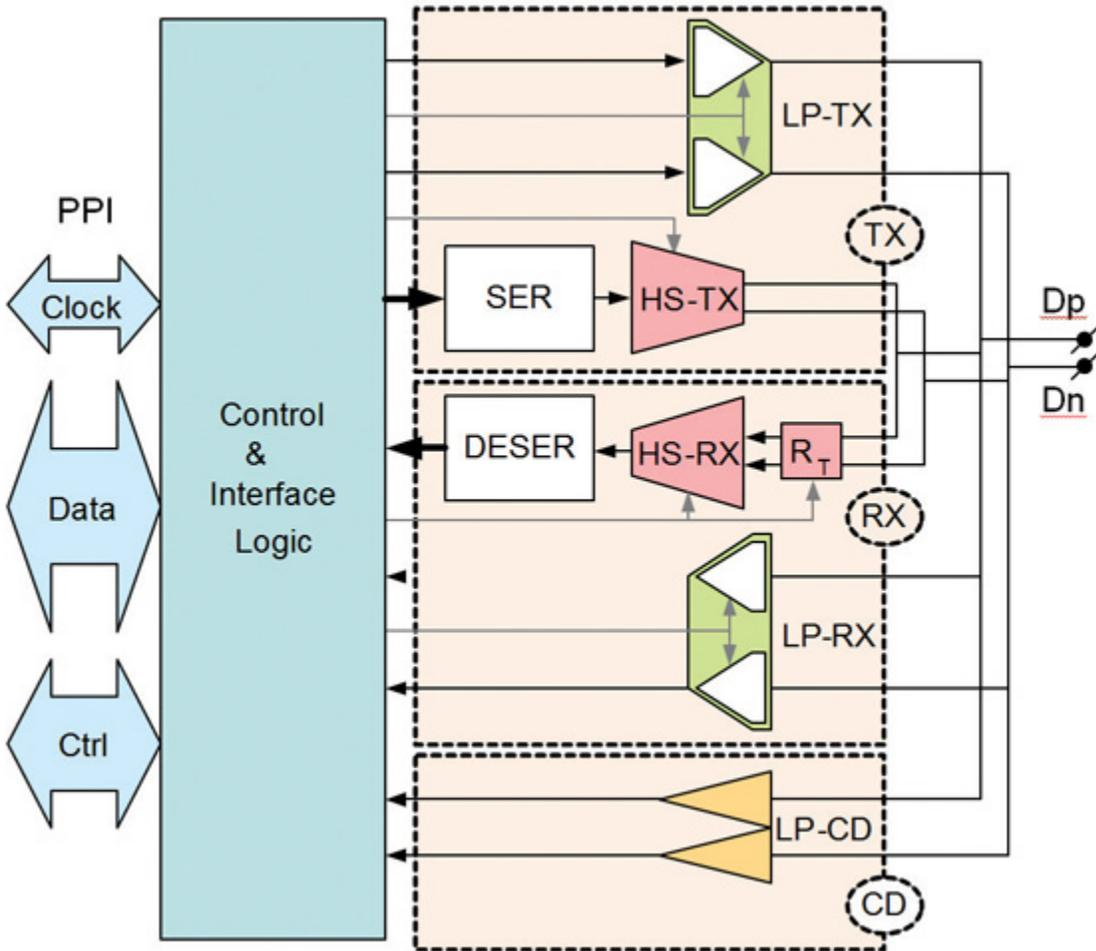
Figure 2: D-PHY Universal Lane configuration supports testability at the expense of large overhead
