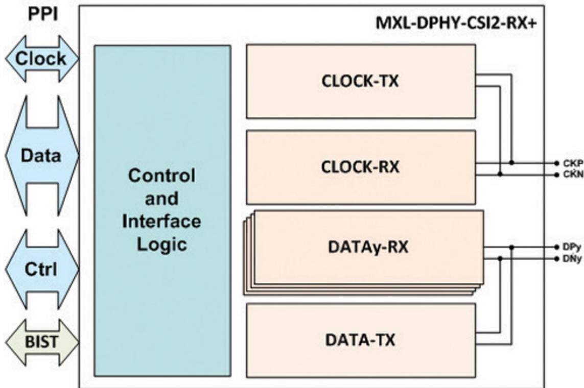
Figure 4: Mixel's RX<sup>+</sup> optimized configuration
