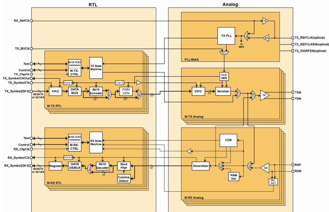
**Figure 1 - Block Diagram of fully featured M-PHY**
